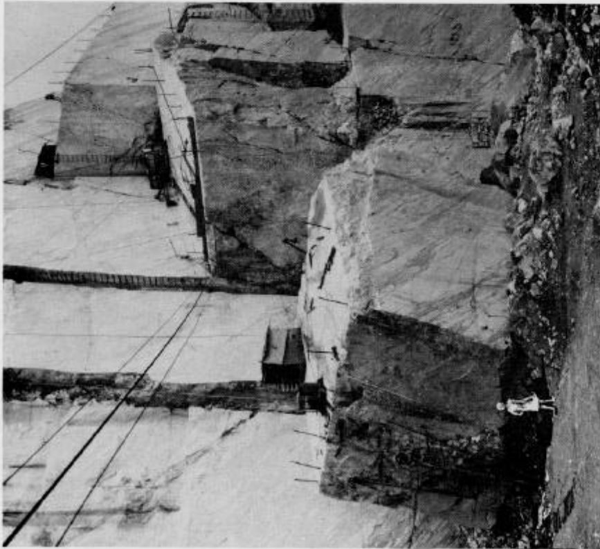
a. Large block, the result of primary extraction by means of a running wire saw. It comes from the sloping platform above and behind it
