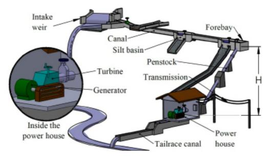
Figure 1. Components of an MHP plant (Culaba & Marfori 2020).
